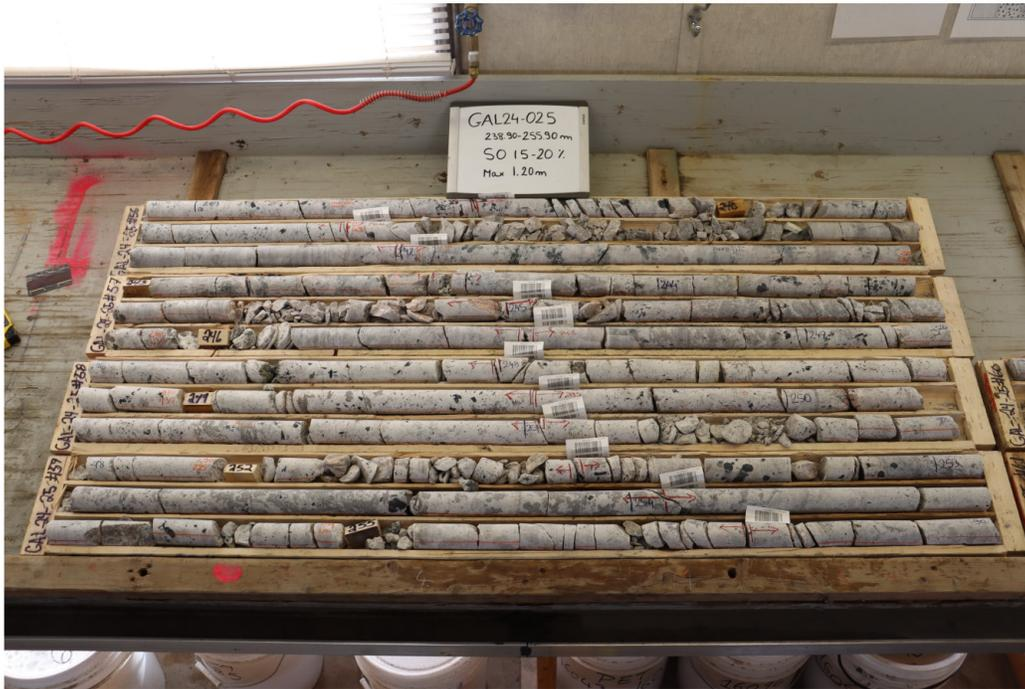
**Photo 4:** Wide spodumene pegmatite interval with coarse spodumene in Hole GAL24-025 (this picture: from 238.9 m to 255.9 m).
