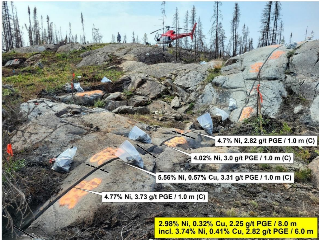
Photo 1 - Channel 1 (view to the southwest) : total horizontal length of 12.0 m, 1-m long channel samples, results of 4 samples reported on this picture.
