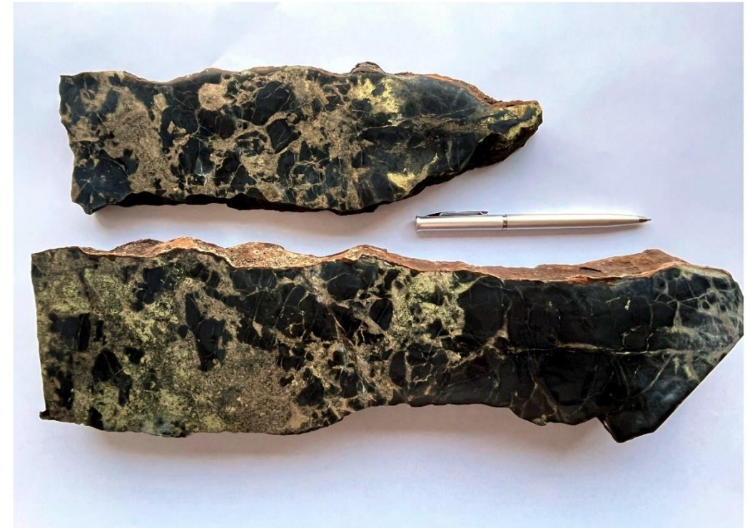
Photo 2 - Semi-massive mineralization with pentlandite, chalcopyrite and pyrrhotite in brecciated ultramafic volcanics.
