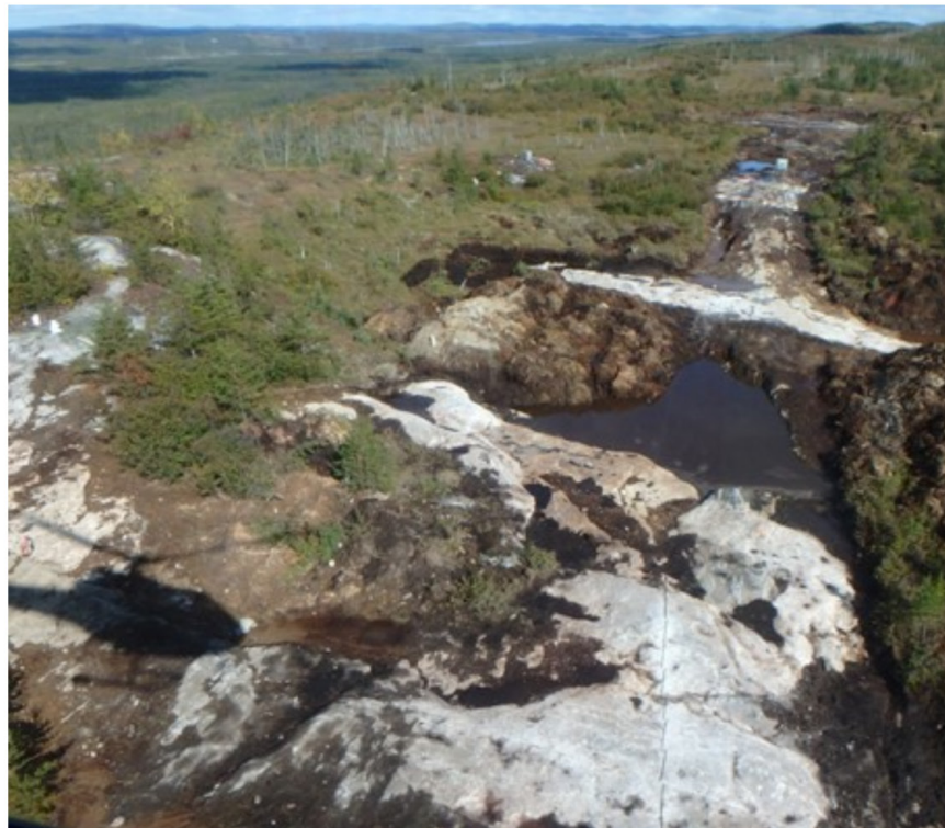
Photo 2 - Lithos North area (looking east). Mechanical stripping significantly extending known pegmatites and uncovering new ones.
