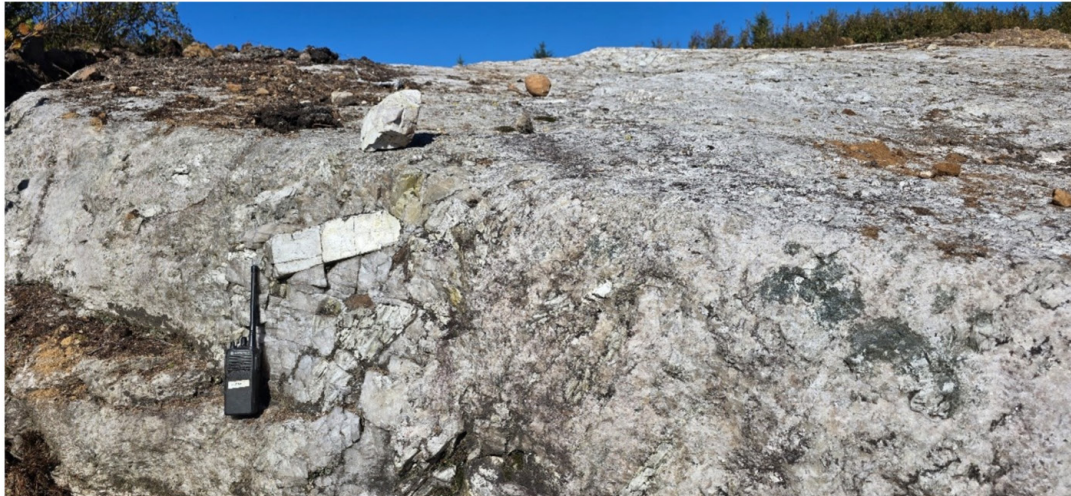
Photo 3 - Lithos North (Pierrot sector). Massive pegmatite body with very coarse whitish spodumene crystals.
