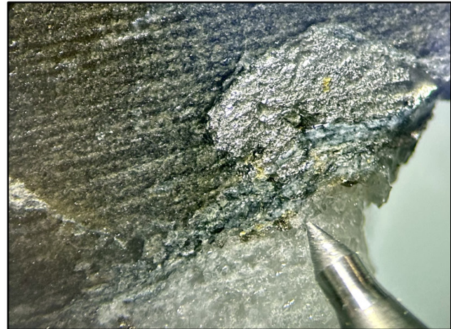
Photo 2 - Hole WR26-45 at 160.1 m. Native gold grains on the edge of arsenopyrite in a quartz vein hosted in tuff metavolcanics. Sample 2436675: 4.01 g/t Au / 1.5 m (from 159.0 m).
