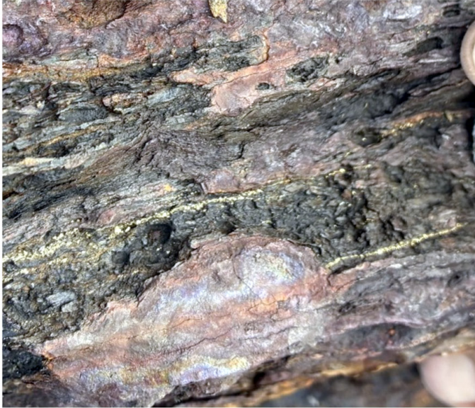
Photo 5 – Livia Showing – Silicified basalt with chalcopyrite stringers (pending results).
