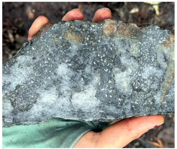
Photo 8 – Ginger showing – Arsenopyrite and quartz veins hosted by metasediments. Up to 3.71 g/t Au (grab sample).
