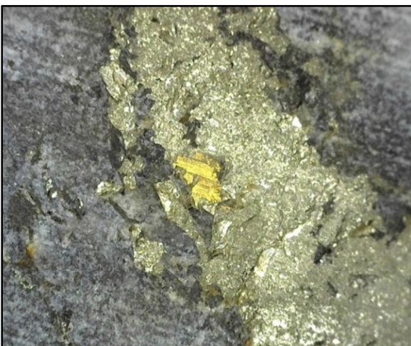
Photo 3 - Native gold, pyrite and quartz at 732.58 m along core (643.9 m vertical depth).
